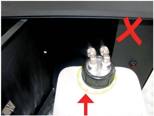
When placing the fluid can into the FLAMANIAC like this, the fluid hose will fold. A folded hose will cause damage to the pump of the unit. **NO GUARANTEE!**
